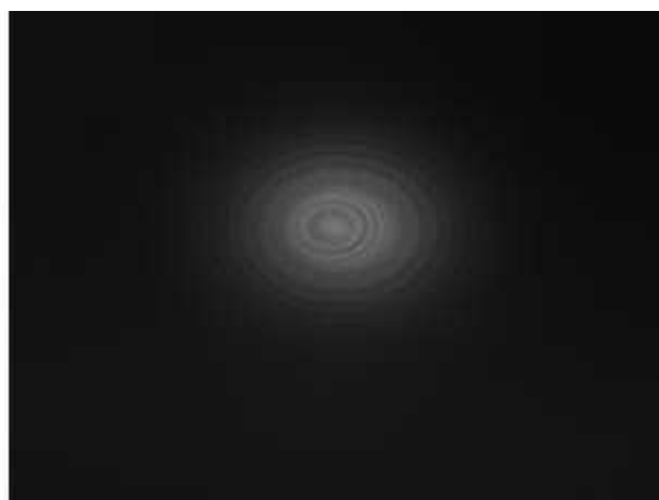
Light emerging from a single mode fiber
